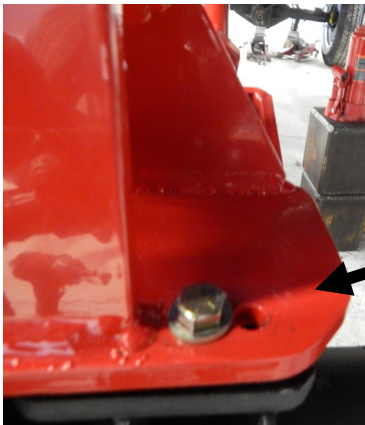
Passenger side uses hole closest to the tire. Opposite of the drivers side.
