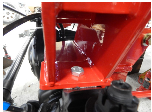
Passenger side uses hole closest to the tire. Opposite of the drivers side.
