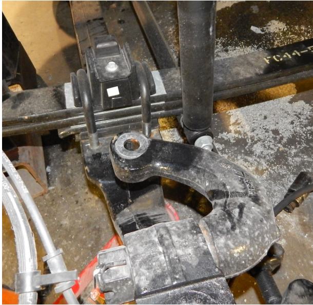
The radiator bolt in gusset removed on drivers side
