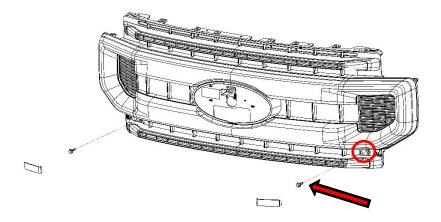
**3**: Remove the six screws across the top of the grille, these will be reinstalled. Remove the two nuts located on the back side next to headlight. Disconnect the camera wiring and camera washer fluid tube if equipped.
