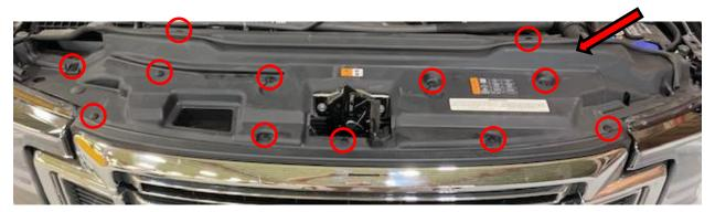
2: Remove the two lower corner screws, these may be located behind trim. The trim is clipped in place, pull forward to remove.
