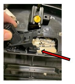
**6**: If installing a light equipped Kelderman grille removed the horn bracket and remount it on the corner gusset. **NOTE:** Moving the horn is required for light clearance.
