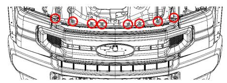
**4**: The remainder of the grille is held in with clips carefully pull straight forward at each clip location to remove the grille from the truck.
