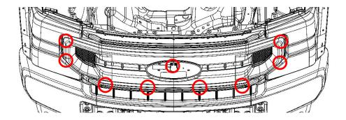
**5**: Remove the two screws that hold the camera washer to the back side of the grille to access the camera. The camera will be reinstalled.
