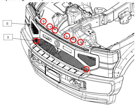
**9:** Use the OEM hardware removed in *step 1* to reinstall the black plastic radiator cover panel. NOTE: Carefully shut the hood while checking the clearance between the hood and the radiator cover panel, adjust the panel if required.
