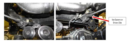
**5:** Fasten the side plate (2) and the panhard bar crossmember (12) to the bottom frame rail flange using 1/2" hardware (10, 11, 15, & 16).
