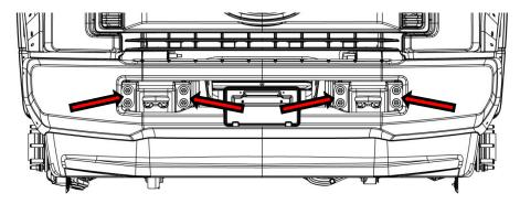
**4:** Remove the eight bolts that fasten the upper bumper brackets and tow hooks to the frame. Remove the four bolt tabs that fasten the lower bumper brackets to the frame. The four bolt tabs will be reused during installation.
