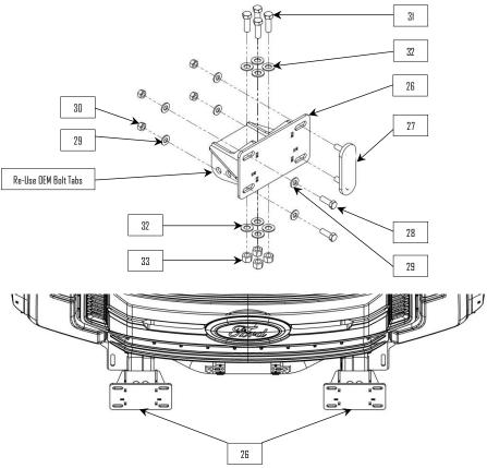
1: Install the bumper frame brackets (26). Use the provided 9/16" bolts, nuts and washers (31, 32 & 33) to bolt thru the top of the frame. Re-use the bolt tabs from step 4 in the "Bumper Removal" section to bolt thru the sides of the frame.
