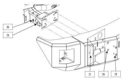
**2:** Use the studs of the bumper mount bolting tabs (27) to position the bumper on the frame brackets. Use provided  $\frac{1}{2}$  washers and nuts (29 & 30) to fasten the bumper to the mount.
