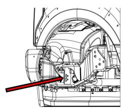
**3:** With the bumper supported remove the two covers on each of the tow hooks and remove the eight bolts. The bumper can now be removed.
