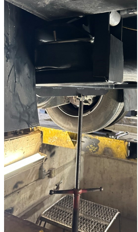
Spacers and Hat Bushings stacked on outer side of tapered shackle
