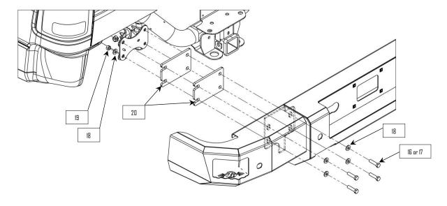
**9**: Align the bumper on the truck and tighten the mounting hardware.
