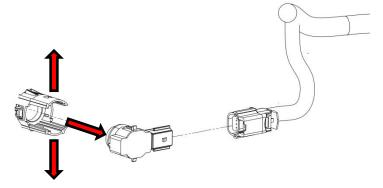
**6**: Depress the tabs on the sensor bezel and push it thru the front of bumper.
