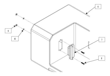
If optioned, install the reverse lights into the center section.
