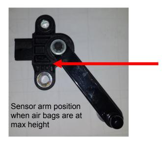
Make sure to have 1/8" gap between the sensor arm and the stops when air system is maxed out as well as fully dumped
