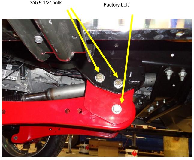
4. Remove the steering arm from the stock pitman arm. Set aside the nut, locking crown and cotter pin. Now remove the pitman arm. You will reuse the nut and lock washer. Next remove the pan hard bar bolt and pan hard bar mount. Locate and install the drop pitman arm (part# FA 450). Torque the factory nut to 275 ft/lbs and torque the steering arm ball joint nut to 115 ft/lbs. Reinstall the locking crown and cotter pin. NOTE: After 15 miles re-torque the pitman arm.
