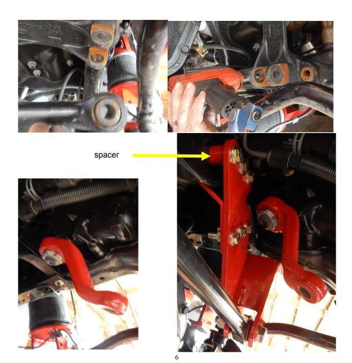
5. Locate the pan hard bar (track bar) drop bracket (part# 16847) with backing plate, (part# 15381). Install the pan hard bar drop and backing plate with the supplied bolts and spacers. Use the pictures below for bolt placement. NOTE: The button head bolt goes in the hole closest to the air bag. Make sure the smooth head is on the bottom of the frame with the nut and threads on the inside of the frame. Torque the M20 bolt to 150 ft/lbs and the 1/2" bolts to 85 ft/lbs
