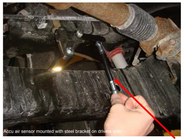
The sensor linkage can be shortened. Just remove the female connector off the rod as well as the jam nut. Then remove the black sleeve. The threaded rod can be shortened if needed. The Accu air sensor can be mounted like the Hadley valve is on the previous page.
