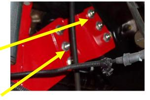
These three bolts are 1/2x3 install the spacers between engine cross member and pan hard bar mount.
