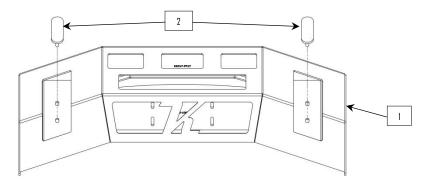
Install the tow hooks (6) into the pockets using the provided 7/8" hardware (3, 4 & 7). Tow hooks (6) and rubber washers (5) go inside the pocket. Tighten the 7/8" nut (7) to the point where the tow hook will still spin, but not freely.
