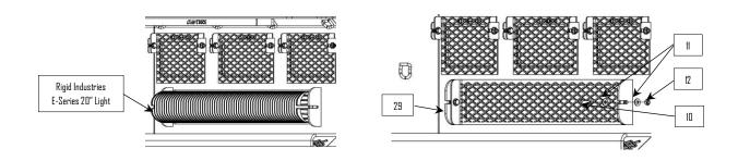
Bolt the end caps (14 & 15) onto the center section using the supplied hardware (16, 17, & 18). Re-positioning may be required after bumper is installed onto truck. **NOTE**: While positioning use masking tape to protect painted surfaces that come into contact.
