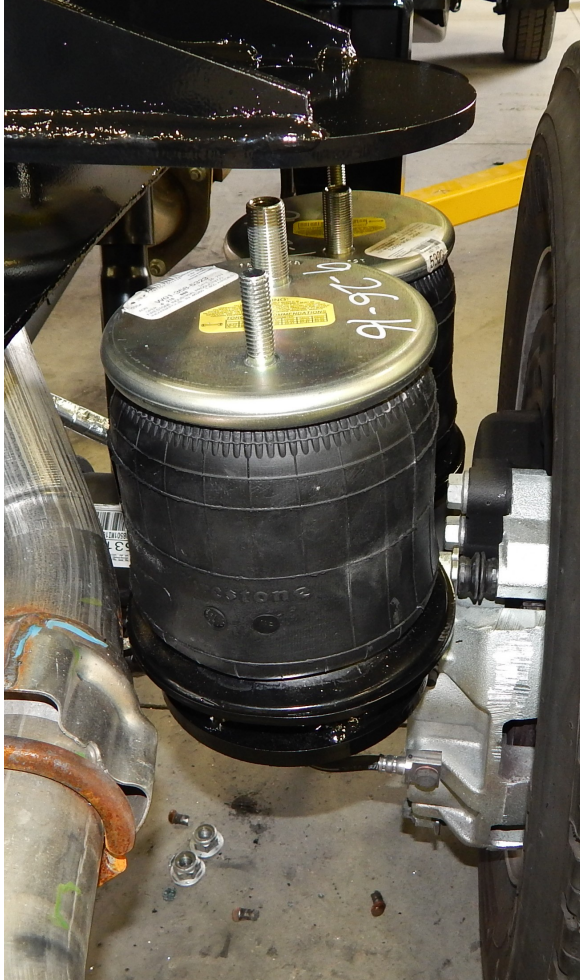
Nut faces the wheel on the rear trailing arms
