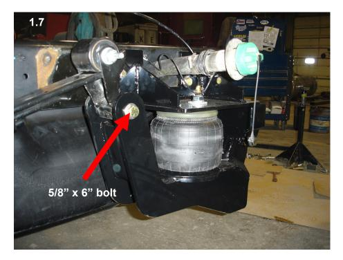
Locate the 5/8" x 6" bolts. Use these bolts to fasten to the leaf spring shackle. Make sure you have a flat washer on each side. Snug up the bolts. Do not torque these bolts (1.8). If you do the suspension system will bind and will not work correctly.
