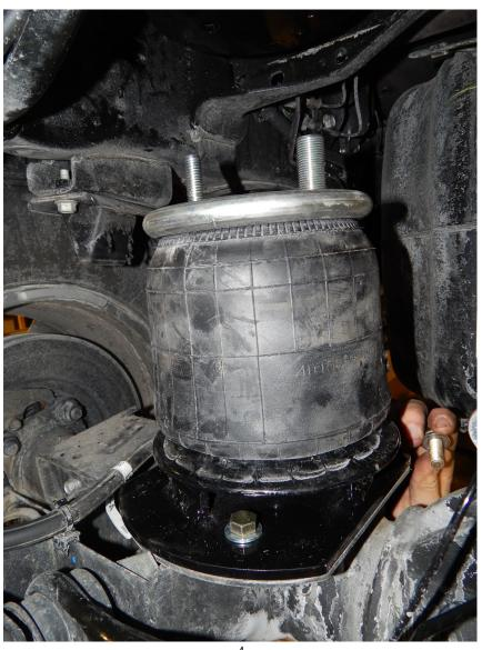
6. With the air suspension is installed, re-connect the factory end links to the sway bar and re-connect the lower shock bolt.
