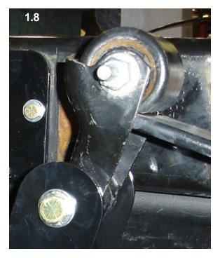
10.Go back and snug up the 5/8" x 5" bolt that holds the swing arm in place. As in step 9, do not torque or the suspension will bind.
