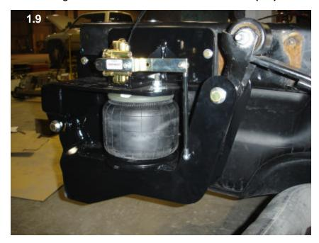
12. Operation. Inflate the air bags so that they are between 6 1/2-7" tall. The other indicator of operation height is to inflate the bags so that the bottom swing arm is level with the ground. As long as you keep the these parameters, the truck will achieve the best ride. When adding a trailer or payload, just add air until the swing arm is level with the ground (2.0).
