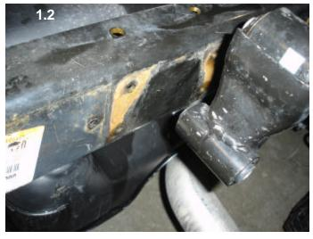
3. Locate the lower 3/8" rear hole in the frame. Use a 1/2" drill bit to drill out the hole in the frame (1.3).
