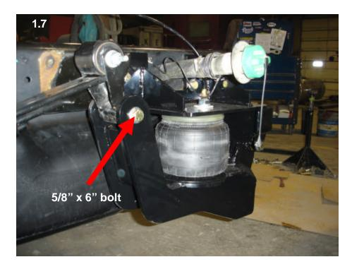
9. Locate the 5/8" x 6" bolts. Use these bolts to fasten to the leaf spring shackle. Make sure you have a flat washer on each side. Snug up the bolts. Do not torque these bolts (1.8). If you do the suspension system will bind and will not work cor-
