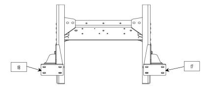
**5**: Use the studs of the bumper mount bolting tabs (3) to position the bumper on the frame brackets (17 & 18). Use washer (20) and nut (21) to fasten the bumper to the mount.
