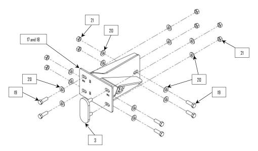
4: Install the bumper frame brackets (17 & 18). Use the supplied 1/2" hardware.
