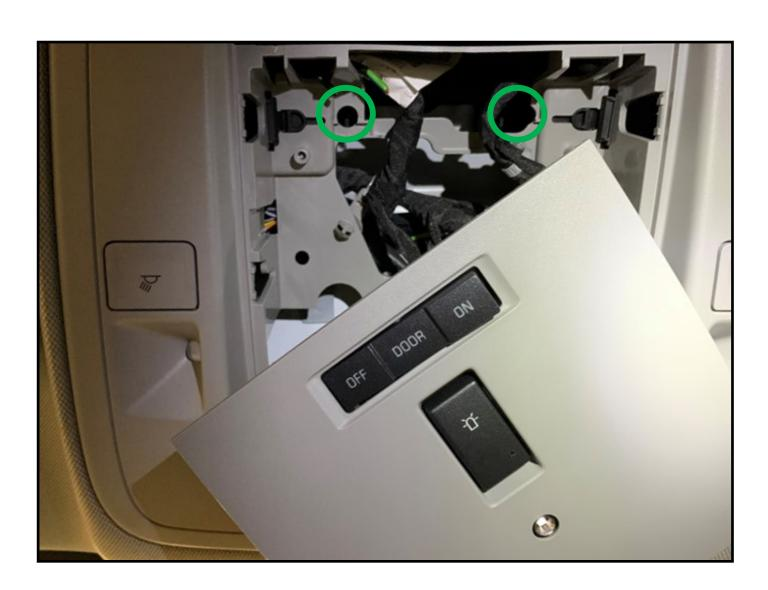
3. Remove the screws circled in green below (2 per side, 4 total) and set aside, these will be used later. Remove the screws circled in red below (2 per side, 4 total).
