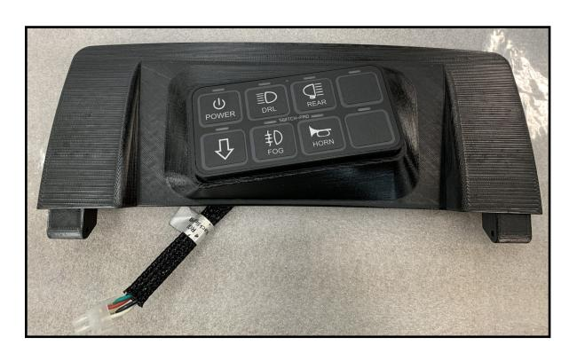
7. Next, slide the mount into the accessory tray cavity and feed the pig tail through the opening on the driver side of the cavity. Secure the mount in place with the screws set aside in Step 2 (take care not to over-torque the screws).
