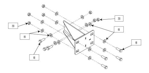
3: Use 1/2" bolts (18) to install the bumper frame brackets (16 & 17).
