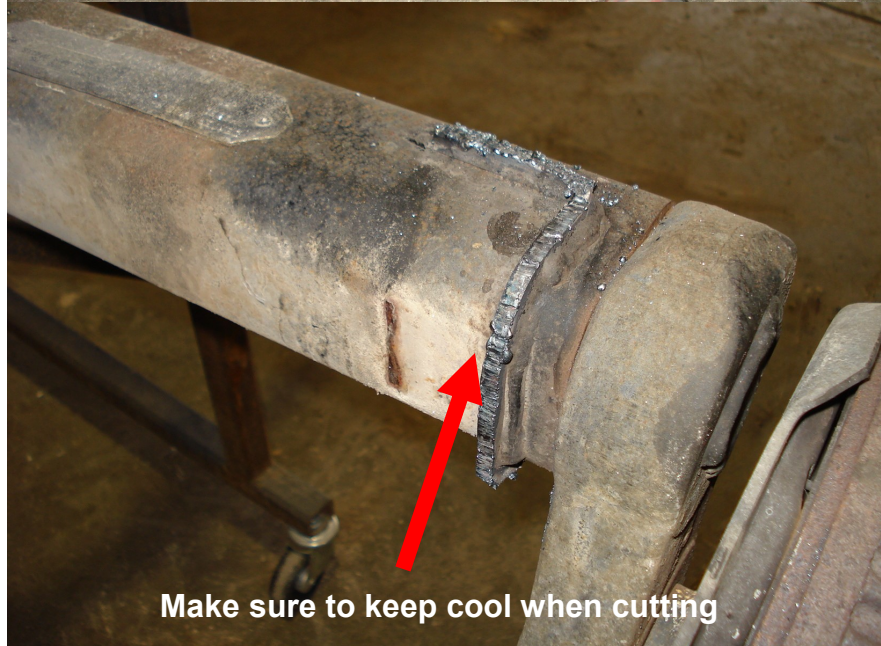
Old brackets cut off the axle
