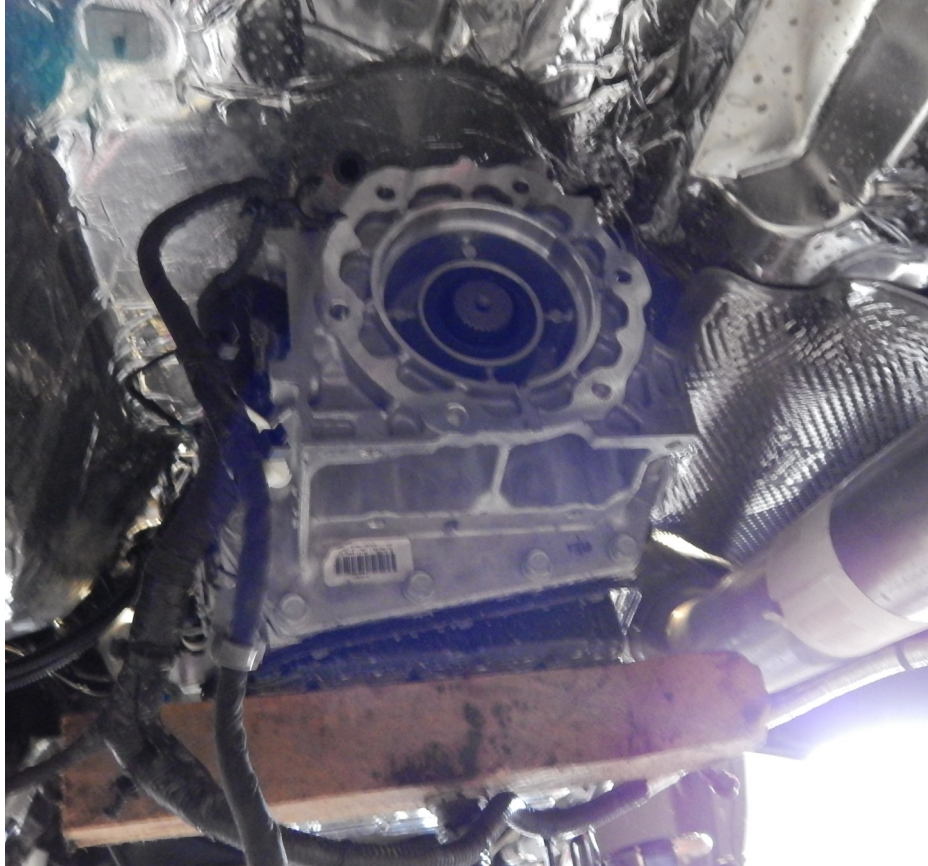
68RFE Pictured above (6 bolt) with Borg Warner transfer case below
