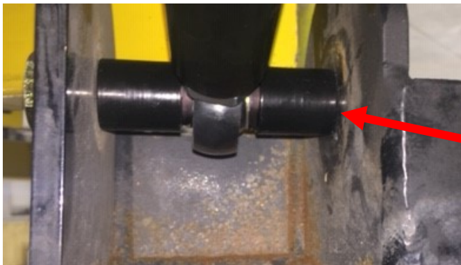
Top trailing arm pictured centered with the machined washers.
