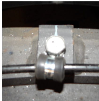
Emergency brake cable bracket bolts to tab on front of air ride cross member
