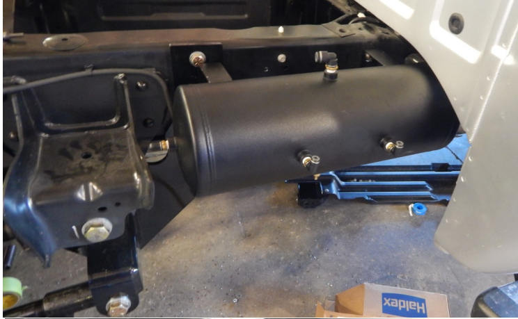
Air tank mounted on the outside passenger side frame rail . The bracket needs to be bent for it to work here. 2 bolts are enough to hold he tank in place
