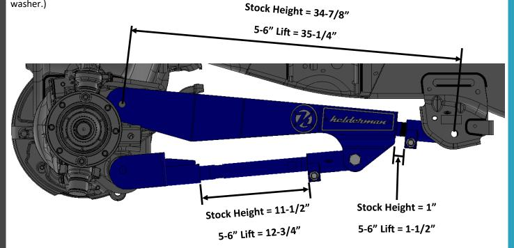
The dimension for each radius should be set to the value above before installation on the truck.
