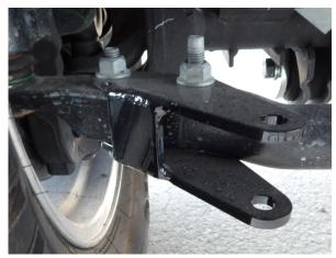
3. Locate the drivers side bracket (part# 18839 and 18397) If fastens to the two factory pinch bolts on the steering arm. It also fastens to the outter tie rod end with the 1/2x3" bolts. Torque these bolts to 55 ft/lbs. Make sure the 1/2" bolt is pointing towards the rear of the truck.
