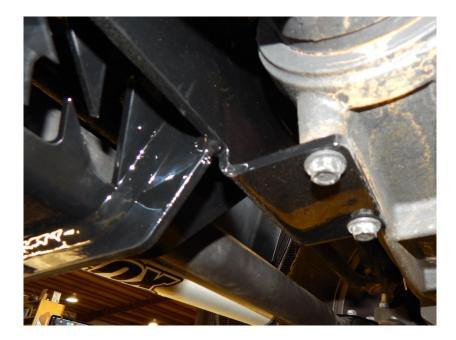
5. Locate the shocks. (Fox part# 985-24-068). Use the 1/2x3" bolts on the outside to fasten the shock to the outter mounts. Next locate the shock strap (part# 18402 and two 1/2x3" bolts. Fasten the shocks to the steering stabilizer bracket. Make sure to put the bolts in top down. Once all the bolts are in place, go back and torque the bolts to 75 ft/lbs.
