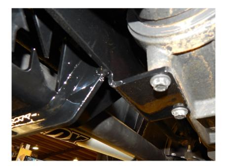
5. Locate the shocks. (Fox Part # 985-24-068). Use the  $1/2 \times 3$ " bolts on the outside to fasten the shock to the outer mounts. Locate the shock strap (Part # 18402 and two  $1/2 \times 3$ " bolts. Fasten the shocks to the steering stabilizer bracket. Make sure to put the bolts in from the top down. Once all the bolts are in place, go back and torque the bolts to 75 ft./lbs.
