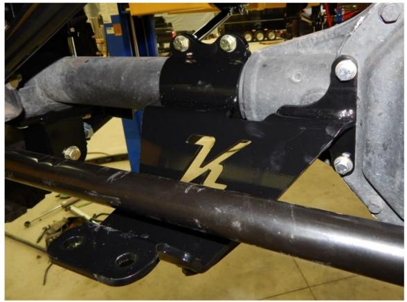
2. Locate the Outer Shock Mounts (#10007481-PS and #30164-DS) and Pinch Plates (#10007483-PS and #30163-DS). The PS Shock Mounts fasten with (4) 5/16"- $18 \times 3$ " bolts to pinch plate. The DS Shock Mount fastens with (2) 5/16"- $18 \times 3$ " bolts to pinch plate.
