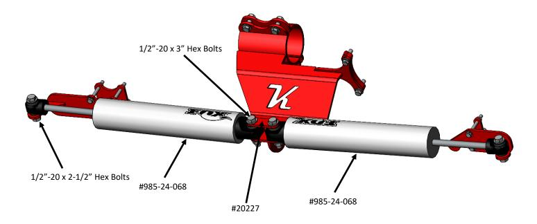
4. Locate with the center bracket and place shock on bracket and install shock strap over shock and drop in (2) 1/2"-20 x 3" bolts. Follow procedure with second shock. Tighten these bolts to 85 ft/lbs.
