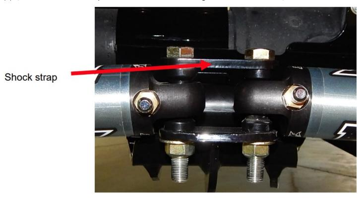
5. Place shock end on the topside of each end shock weldment and drop in (1) 1/2"-20 x 2-1/2" hex bolt on each side. Tighten these bolts to 85 ft/lbs.
