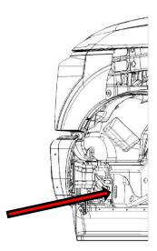
3: With the bumper supported, remove the four bolts located on either side of the two tow hooks. The bumper can now be removed.
