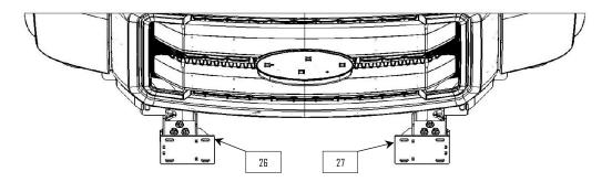
7: Use the studs of the bumper mount bolting tabs (3) to position the bumper on the frame brackets (26 & 27). Use washer (29) and nut (30) to fasten the bumper to the mount.
