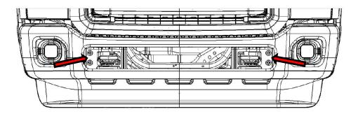
4: Remove the six bolts that fasten the tow hooks to the frame. These will be reused during install.
