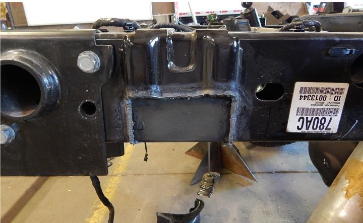
7.) Trimming of the rear bumper mounting brackets is required to install the rear air suspension. Locate the factory rear bumper and remove the corner bracket. It will not be re-used.
