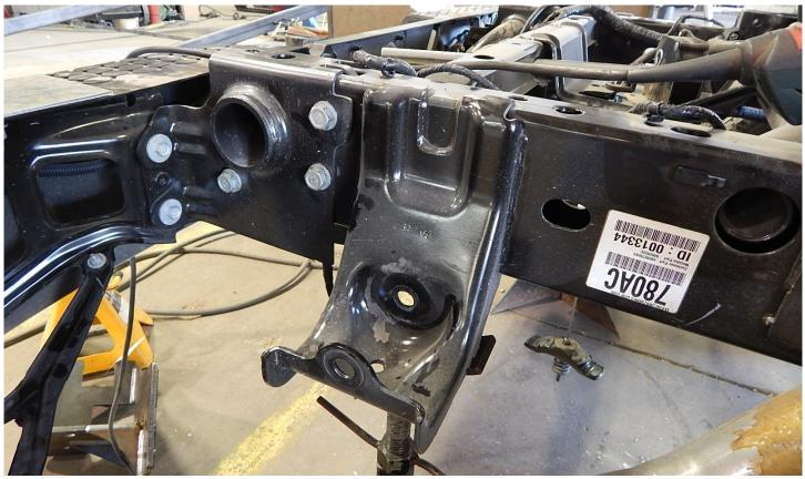
6.) Using a torch, saw or a plasma cutter, remove the shackles from the frame as shown in the photo below. **DO NOT CUT INTO THE FRAME.** The leaf springs do not have to be removed for the installation of this kit.
