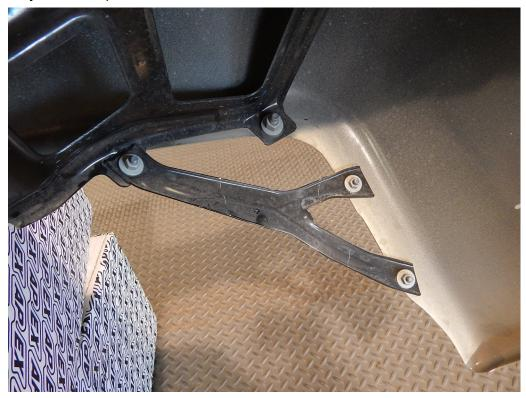
8.) Mark each side of the inner bumper mounting structure as shown in the photos below.. Use a cutting wheel to cut off the part of the structure that needs removed. Take your time while cutting and be sure not to cut into the bumper itself. The entire substructure of the rear bumper can also be removed if you do not wish to cut it.
