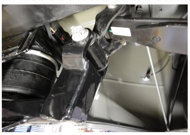
13.) Locate the 1/2 x 3 /12" bolts, flat washers and lock nuts. Insert the bolt through the bottom of the swing arm and up through the bottom of the airbag. You may need to wiggle the bottom of the airbag side to side to get the bolt to align properly in the threads of the airbag. With the bolt started in the threads, torque the bolt to 30 ft./lbs. **DO NOT OVERTIGHTEN THE BOLT OR IT WILL CAUSE DAMAGE TO THE AIRBAG.**
