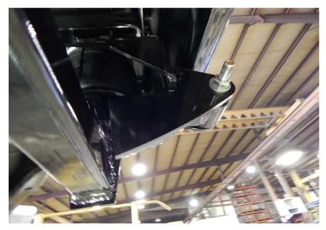
12.) Slide the swing arm up so that the ears of the swing arm. It might be necessary to raise or lower the truck using the jack to get everything lined up properly. Once the swing arm ears line up with the shackle hole, connect them with the shackle bolt removed from the truck in step 4. **NOTE: The shackle bolt needs to be installed from the inside out with the bolt head near the frame side.**
