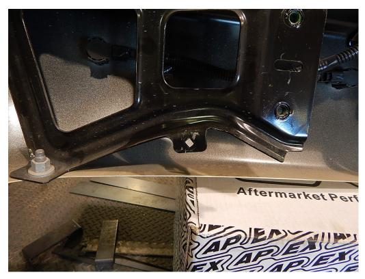
9.) With the leaf spring perches removed, locate the upper framework of the 2-Stage Rear Air Suspension. Remove the (3) factory 14mm bolts from each side of the factory hitch framework. The upper framework will fasten into the frame/hitch assembly with these 14mm x120 bolts. Torque these bolts to 115 ft./lbs.
