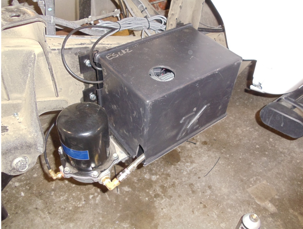
Upper forward mount fastens to the box mount closest to the cab on long box
