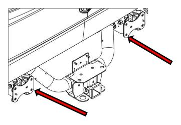
**5**: If equipped remove the parking sensors from the stock bumper **NOTE**: Keep track of location. Spread the ears on the sensor bezel and push the sensor thru the back of the bumper.
