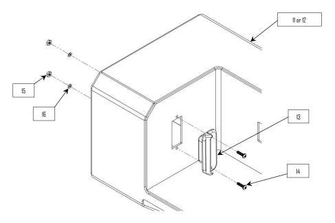
If optioned, install the reverse lights into the center section.
