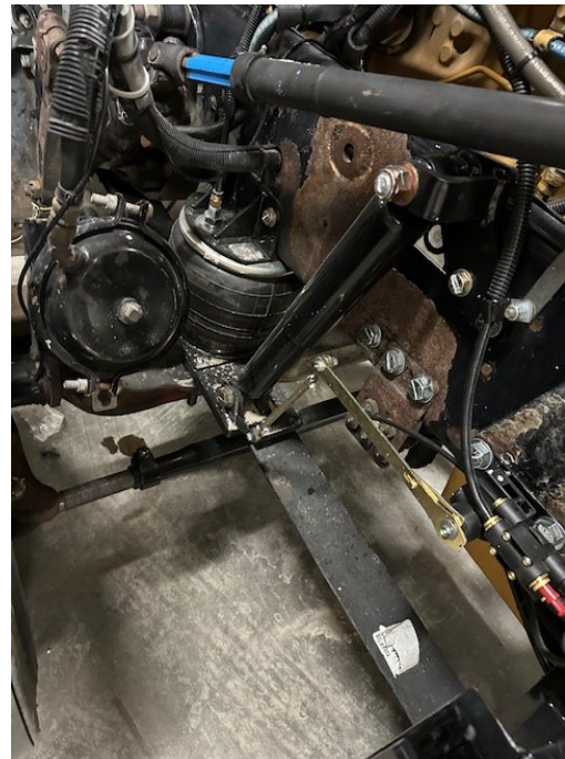
Figure #13: Shows the approximate angle of the shock. Also the position of the height control valve mount on outside of shock mount
