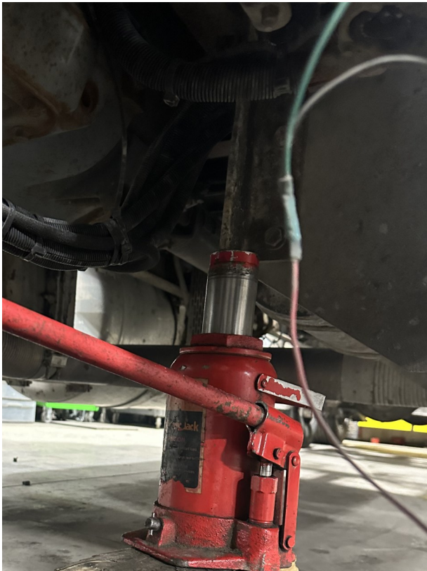
Figure #1-3: shows approximate locations of jacks front dot is on frame or strong points of truck.
