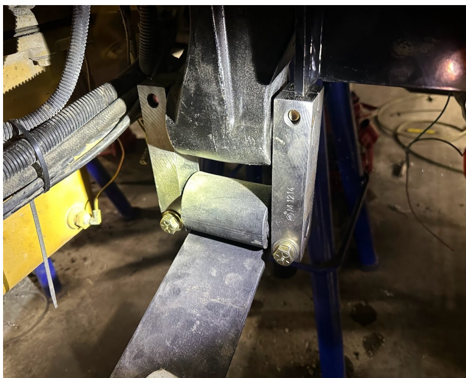
Figure #6: Shows Rear Leaf spring assembly with shackles attaching the leaf to the casting mount.
