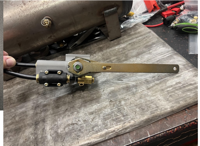
Figure #11: Passenger side orientation of height control valve. ( Note: This will comes with a plug for the passenger side only )
