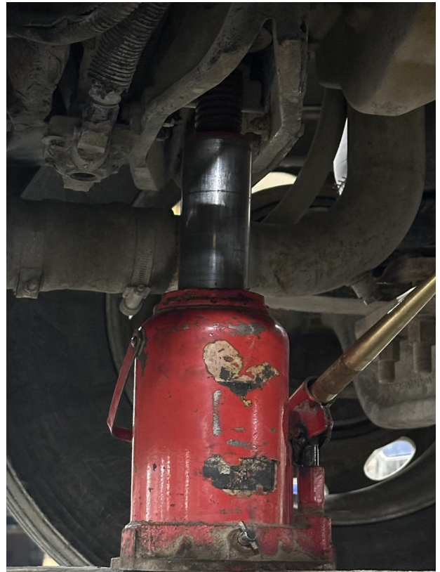
Figure #1-3: shows approximate locations of jacks front dot is on frame or strong points of truck.
