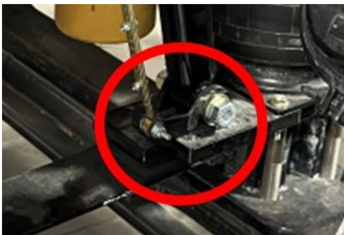
Figure #14: Figure shows height control valve assembly and lower mount for height control valve attached to the lower bag mount.
