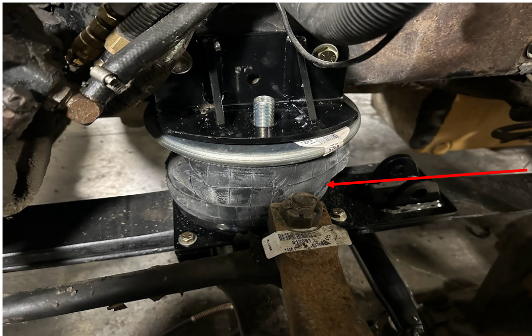
Figure#9 : Bag is bolted to the lower bag mount with the stud facing out. Top bag mount is installed using two bolts "You will need to use a grinder to smooth the edges of the steering arm to allow for extra clearance"
