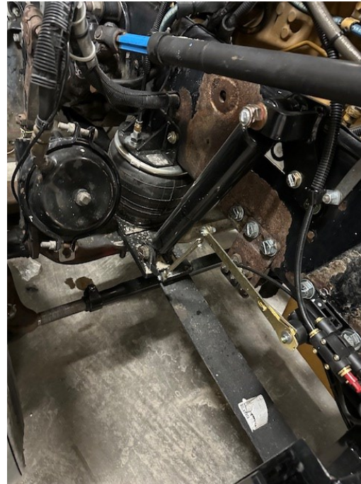
Figure #15: Shows the approximate angle of the shock. Also the position of the height control valve mount on outside of shock mount
