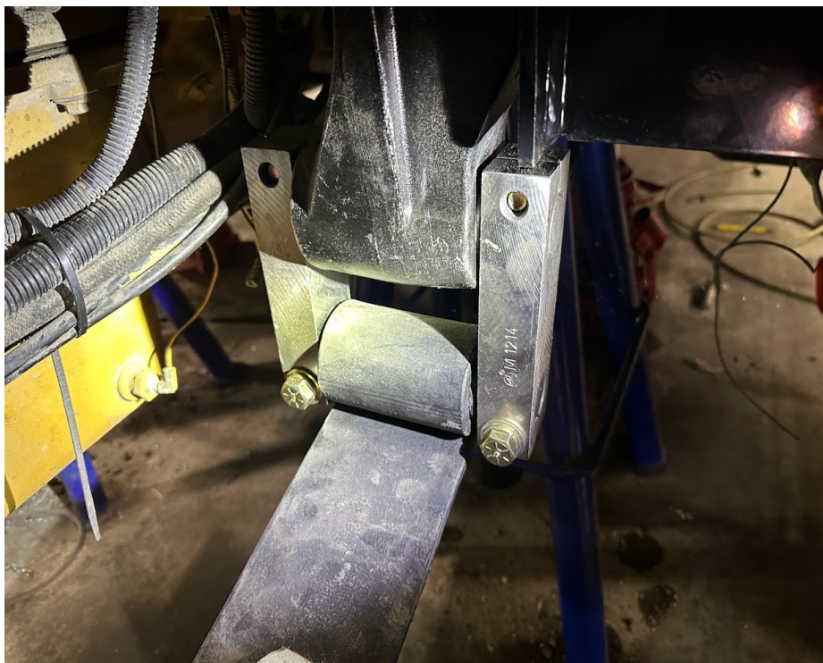
Figure #7: Shows Rear Leaf spring assembly with shackles attaching the leaf to the casting mount.
