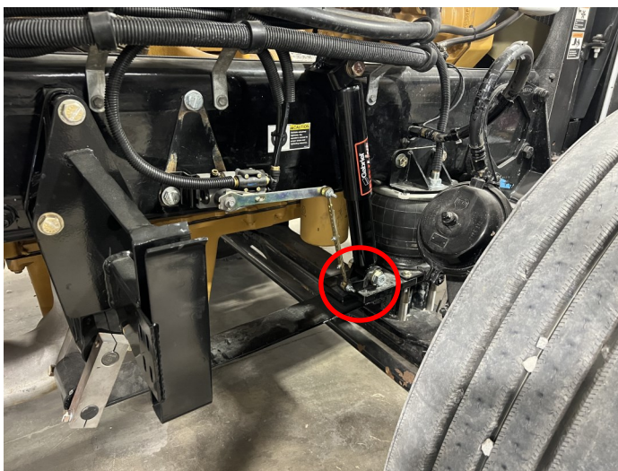
Figure #16: Figure shows height control valve assembly and lower mount for height control valve attached to the lower bag mount.
