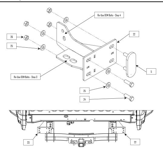
**8:** Install the bumper frame brackets (22 & 23). Re-use the hardware removed in steps three and four.
