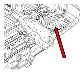
**3**: Remove the bolt tab from each side that fasten the bumper bracket to the frame. Save these as they will be re-used later when installing the new brackets.
