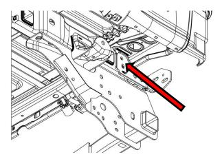
**4**: Remove the bolt tabs from each side that fasten the bumper bracket to the tow hitch. Save these as they will be re-used later when installing the new brackets. The bumper brackets can now be removed.
