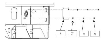
Bolt the end caps onto the center section using the supplied 3/8" hardware. Position the tops flush with the center section. NOTE: while positioning use masking tape to protect painted surfaces that come into contact.
