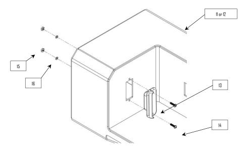
If optioned, install the reverse lights into the center section using the hardware supplied with the light.
