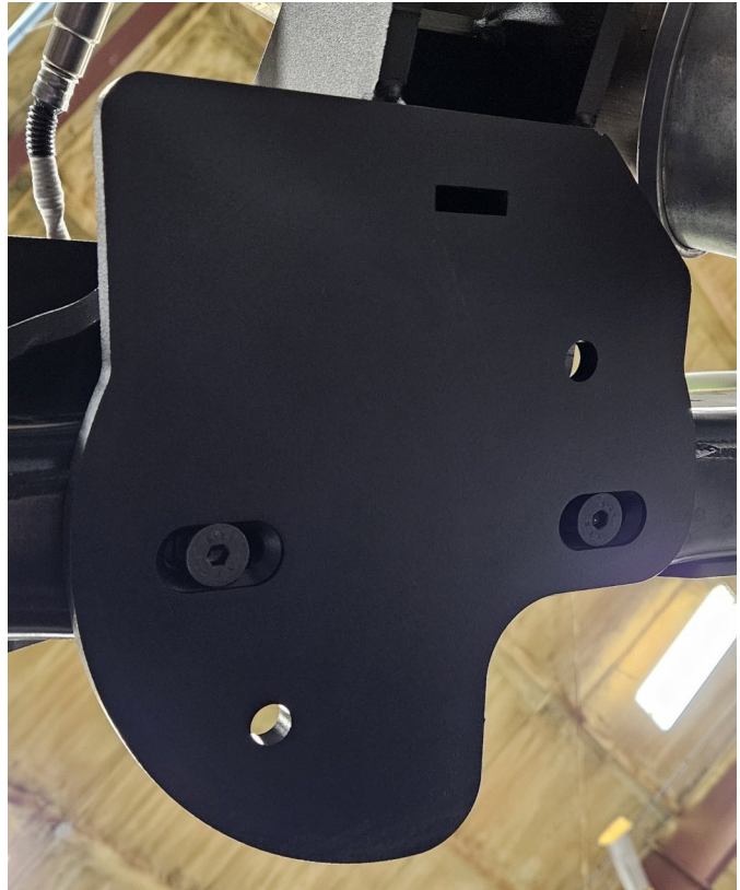
Drivers Side shown with M10 bolts installed.
