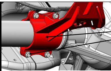
NEXT YOU WILL WANT TO INSTALL THE AXLE CLAMPS USING THE 7/16" HARD WARE. NOTE: YOU WANT TO ATTACH LOOSELY UNTIL YOU TIGHTEN THE DIFFERENTIAL COVER BOLTS.
