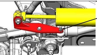
FIRST, YOU WILL WANT TO LIFT THE TRUCK ON A LEVEL SURFACE. THEN REMOVE THE OUTER DRAG LINK BOLTS.
