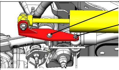
Install the outer shock Brackets using the 5/16"- $18\times3$ " bolts. Then install the factory drag link Bolts.
