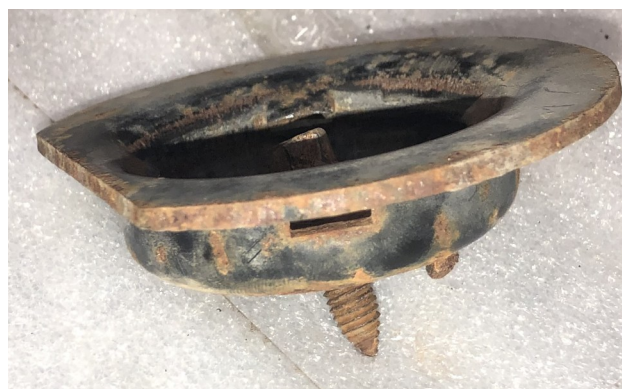
FIGURE 2-3: REMOVE BUMP STOPS BEFORE STARTING THE INSTALLATION PROCESS. REMOVE RUBBER AND THEN UN-BOLT THE METAL STOP PLATE.
