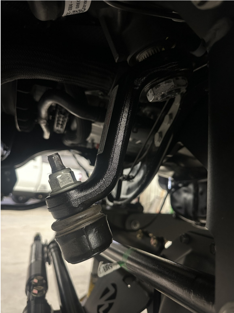
FIGURE 6-7: SHOWS PITMAN ARM INSTALLED
