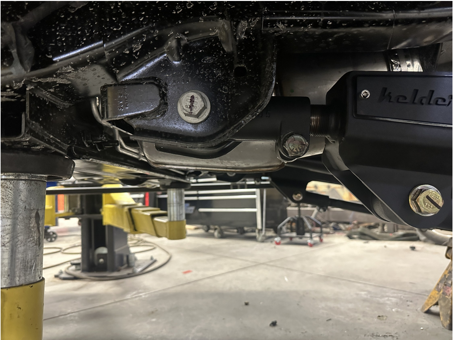
FIGURE 5: SHOWS THE RADIUS ARM INSTALLED IN THE FACTORY MOUNT.
