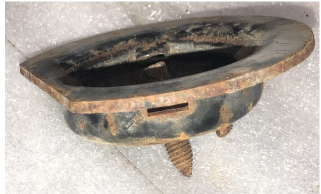
FIGURE 2-3: REMOVE BUMP STOPS BEFORE STARTING THE INSTALLATION PROCESS. REMOVE RUBBER AND THEN UN-BOLT THE METAL STOP PLATE.
