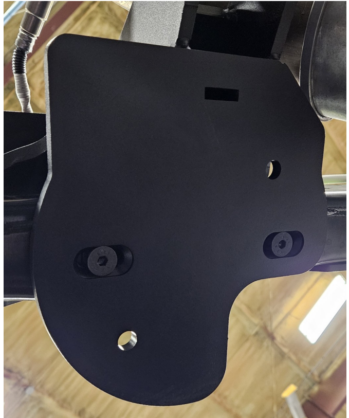
Drivers Side shown with M10 bolts installed.
