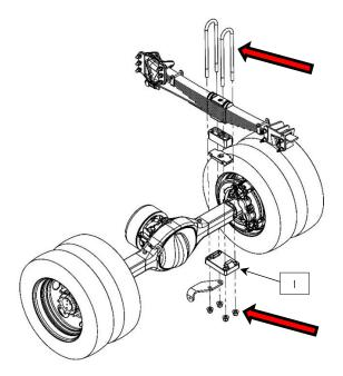
**8**: Remove the pins from each spring hanger and unbolt the leaf spring from the front hanger. The leaf spring is now free to be removed.
