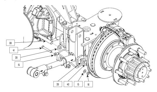
**14**: Once aligned and bolted together tighten down all axle hardware.
