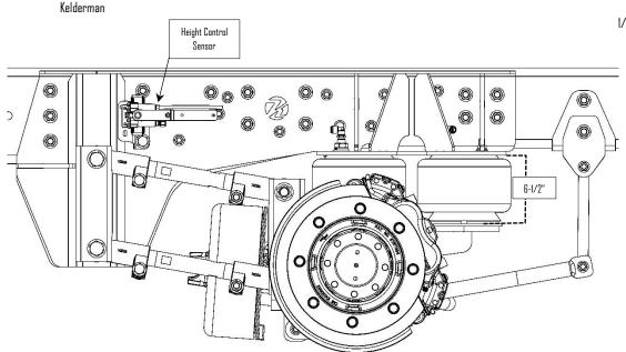
**34**: With the truck sitting at ride height Check pinion angle and wheelbase measurements. Adjust the trailing arm bars as needed to set the rear axle back to factory position. **NOTE:** Refer to notes taken in *Disassembly steps 1 & 2*.
