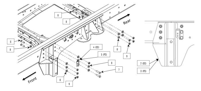
2: Install the upper shock bracket (10) using 5/8" hardware (7, 8, 9, & 11). **NOTE:** Trucks without factory shocks. Use the side plate (2 or 3) as a guide to drill four 11/16" holes in the frame.
