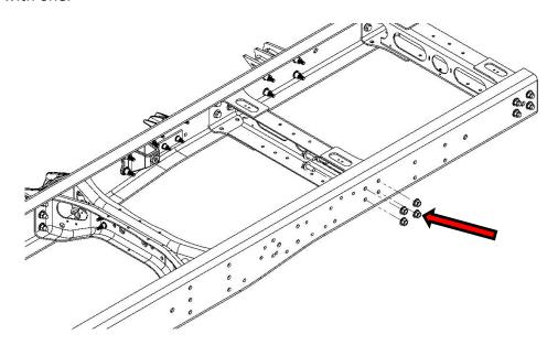
**16**: Proceed to *step 1* of the *Kit Installation* section of these instructions and install the Kelderman side plate onto the now bare frame rail.
