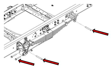
**9**: Mark, measure, and note the frame width at each crossmember. Using those same marks, measure the frame diagonally to check for square. These measurements will be compared against when installing the side plates.
