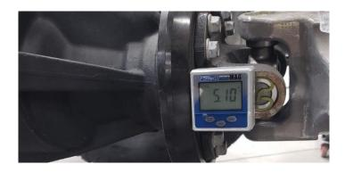
2: Take the following measurements for future reference. These measurements will be used to adjust the suspension after installation.
