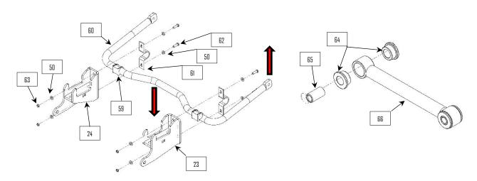
24: Press poly hat bushings (64) and sleeve (65) into both ends of the sway bar end links (66).
