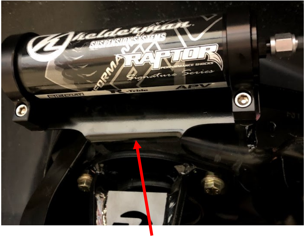
The remote reservoir shock mount fastens in between the upper coil bucket and upper bag mount
