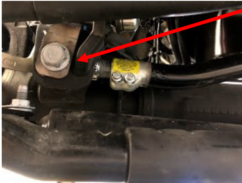
Adjustable track bar installed
