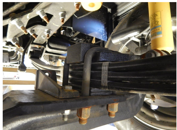
U bolts will be reused
