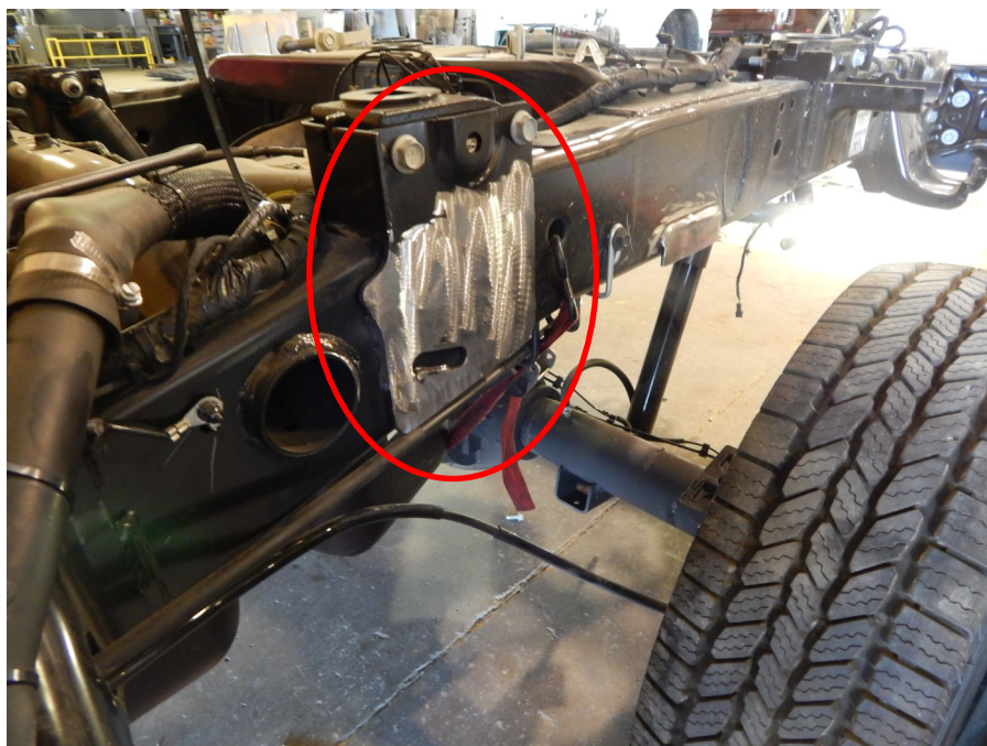
OVERLOAD PERCH SHOWN REMOVED FROM THE FRAME
