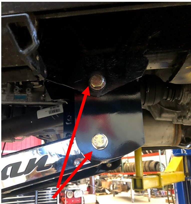
BOLTS SHOWN INSTALLED INTO FACTORY CROSSMEMBER MOUNTS. INSERT BOLTS FROM THE OUTSIDE IN.
