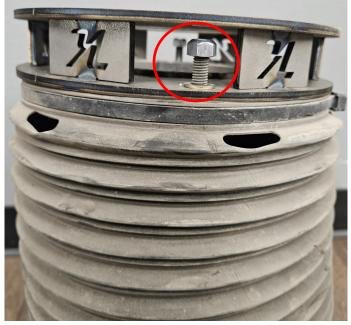
3. Now that the spacer is installed on the air bag, locate the 3/8"-24 x1-1/4" bolts. Use these to bolt the spacer to the axle. Torque to 30 ft/lbs.
