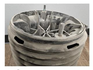
2. LOCATE THE 1.5" RISER (PART# 18477) AND FASTEN IT TO THE BOTTOM OF THE AIR BAG WITH THE M8-1.25MM LOCK NUT & WASHERS. TORQUE TO 30 FT/LBS.
