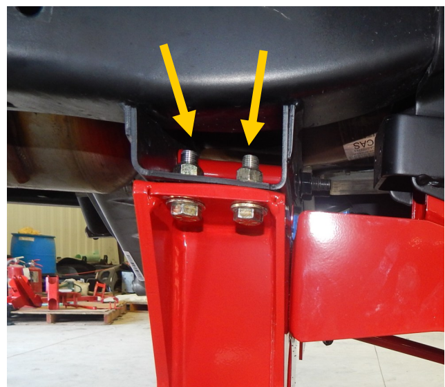
These holes need drilled
