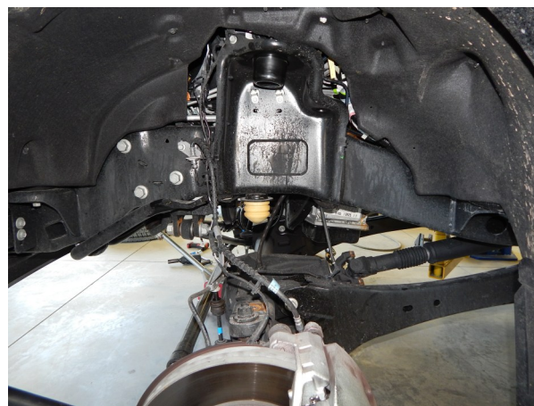
USE THE UPPER AIRBAG MOUNT AS A TEMPLATE BEFORE DRILLING THE HOLES FOR THE 3/8"-24 X 1-1/2" BOLTS
