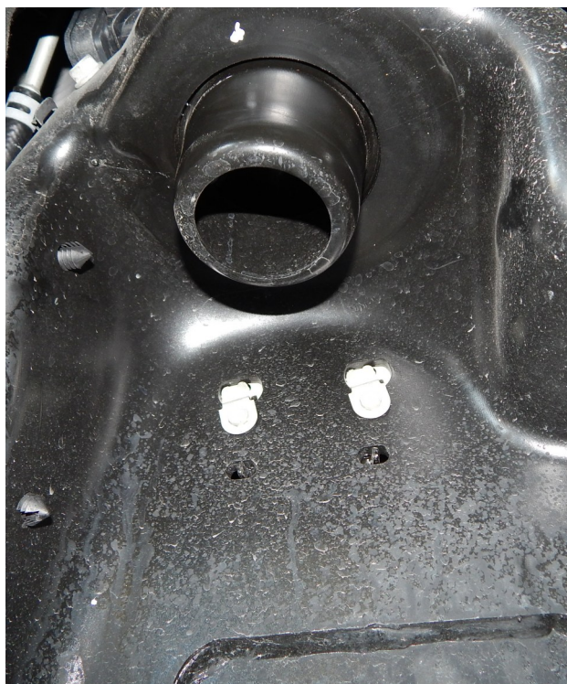
HOLES WILL BE DRILLED FOR THE UPPER AIRBAG MOUNT TO INSTALL INTO THE SPRING PERCH.
