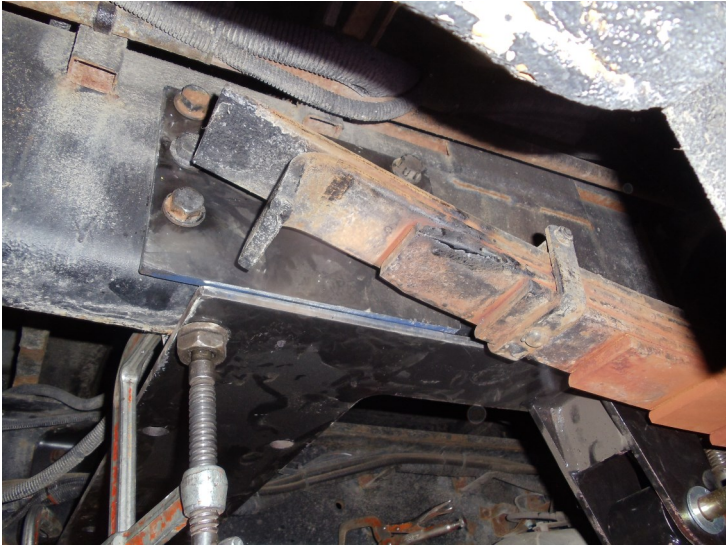
Center the upper air bag holes under the factory crossmember
