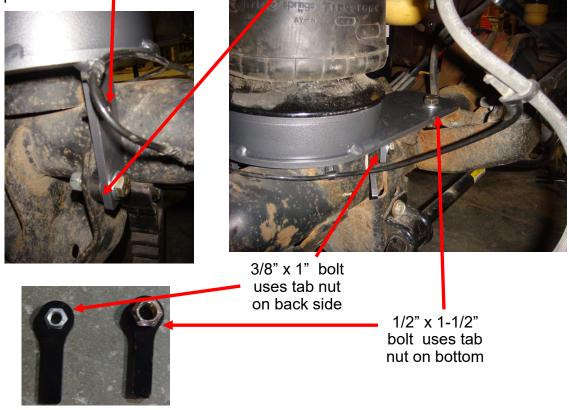
7. Torque the 3/8" bolts to 40 ft/lbs and the 1/2" nuts to 65 ft/lbs.
