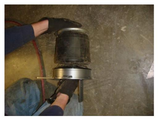
6. Set the Lower Air Bag Mounts on top of the axle They fasten to the axle with the  $3/8" \times 1-1/2"$ , bolts (and Spacer Part# 50789),  $3/8" \times 1"$  bolt and and  $1/2" \times 1-1/2"$  bolts. The  $3/8" \times 1"$  and  $1/2" \times 1-1/2"$  use the tab nuts, being that there is no way to get a wrench on the nuts.
