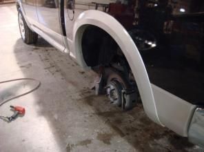
3. Remove the lower shock bolt and disconnect the shock. Lower the axle down until the brake lines are tight. The coils should be loose enough to pull out by hand. Next remove the rubber bump stops. Also remove the plastic mounting tab that holds the wiring for the wheel sensor from the axle.
