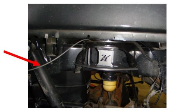
5. Locate the lower air bag mounts (Part #50801-DS and 50802-PS) and 5323 Air Bag (Part #80012-5323). Locate the 1/2" x 4" bolt, lock washer and nut. Snug the air bag to the mounting bracket. Make sure to look at the orientation of the upper bag mounting holes. Make sure to rotate the air bags so that the studs on top of the bag line up with the holes on the upper bag mount. Now you can torque the 1/2" bolt to 30 ft/lbs
