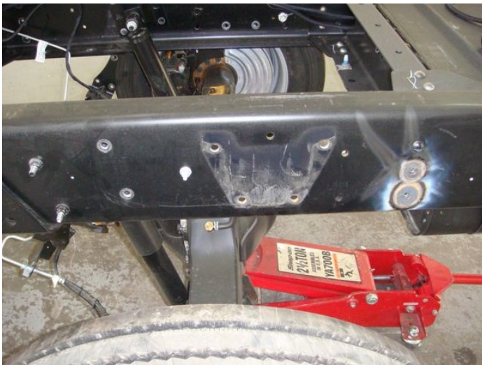
Place jack under axle to keep from rotating.
