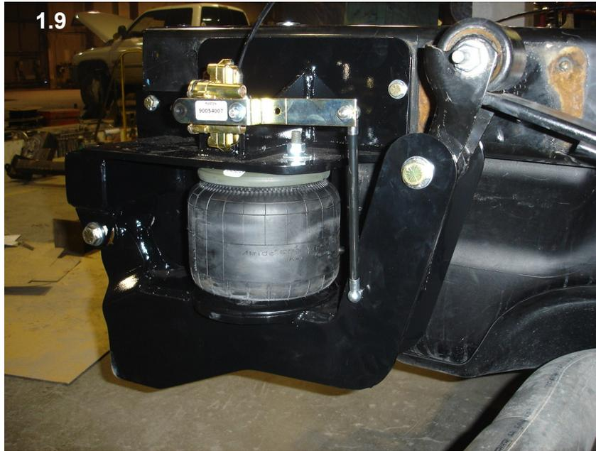
12. Operation. Inflate the air bags so that they are between 6 1/2-7" tall. The other indicator of operation height is to inflate the bags so that the bottom swing arm is level with the ground. As long as you keep these parameters, the truck will achieve the best ride. When adding a trailer or payload, just add air until the swing arm is level with the ground **(2.0)**.
