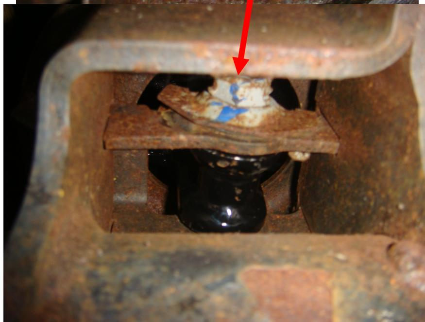
8. Once the lower air bag mount is fastened in place, jack the axle up and fasten the air bag to the upper air bag mount with the 1/2" and 3/4" nuts and lock washers. Torque the nuts to 35 ft./lbs. Locate the air fitting and place in the air port. If your fitting does not have any sealant already applied, apply Teflon tape to the fitting threads.
