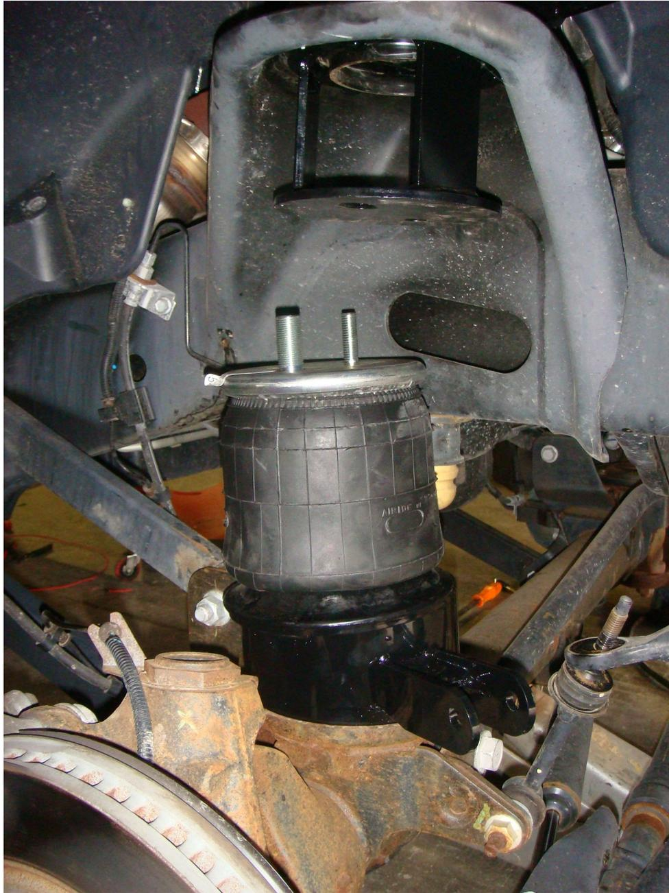
7. Once you have the air bag tightened to the lower bag mount, drop the air bag and lower bag mount into place on top of the axle. Locate the original 14 mm lower shock mount and nut. Wiggle the mounting bracket in place so the holes line up and fasten in place, torquing the 14 mm bolt to 95 ft./lbs.
