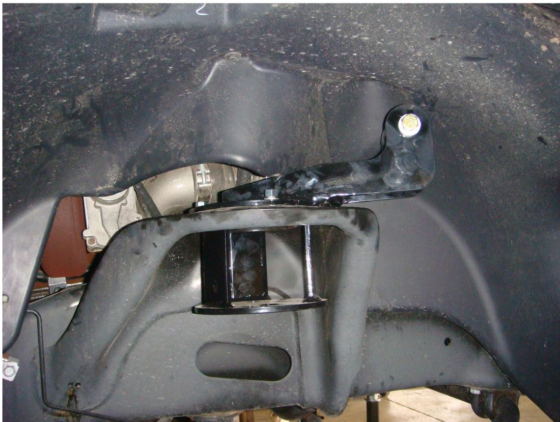
6. Locate the 5323 Firestone air bag. Locate the lower air bag/lower shock mount. Fasten the air bag to the bottom mount with the 1/2 x 3 1/2" bolt and lock washer. Before torquing the bolt, drop the assembly into place and jack up the axle to get the orientation of the top studs of the air bag with the top air bag mount. Once the bag location is determined, torque the 1/2 x 3 1/2" bolt to 35 ft./lbs.
