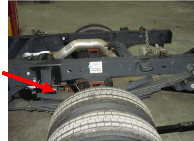
2. On the driver's side separate the emergency brake cables. They will be re-routed through the forward drivers side forward sideplate. Remove the bolt that connects the brake lines to the top of the axle. Also remove the bolt that connects the wiring harness and passenger side e-brake cable to the front side of the axle. These brake lines and cables will now connect to the crossmember of the air suspension. See step 3 in assembly.
