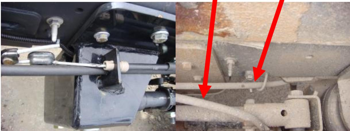
3. Next, remove the front leaf spring perches, leaf springs and factory sway bar end link mounts and the overload pads. Use a torch to cut off the rivets. Next, punch out the rivets.
