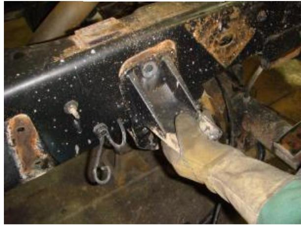
4. The best way to remove the riveted pads is to use a torch to cut the rivet heads off. Make sure that there are no fuel lines, brake lines, or wiring that can be damaged while cutting the rivets off.
