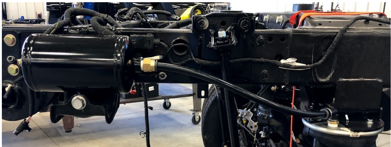
3/4" air line shown installed from airbag to accumulator tanks. Accumulator tanks install with factory rear shackle bolts removed in Step Two.
