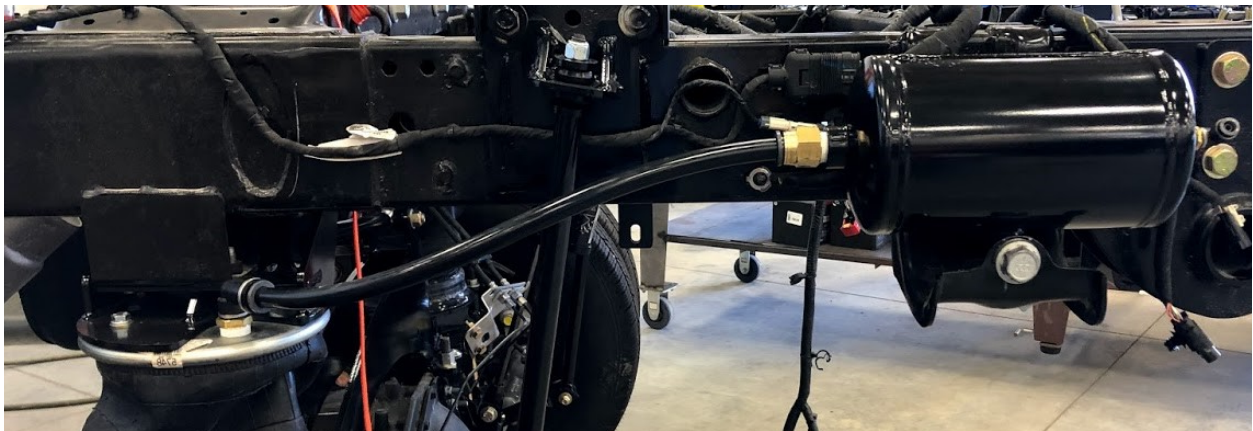
3/4" air line shown installed from airbag to accumulator tanks. Accumulator tanks install with factory rear shackle bolts removed in Step Two.
